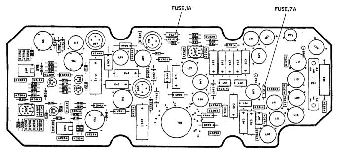
Figure 3-12. Module PS, Fuse Location
