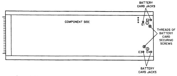
Figure 3-18. Module AUDIO, Component Side, Battery Card Removed
