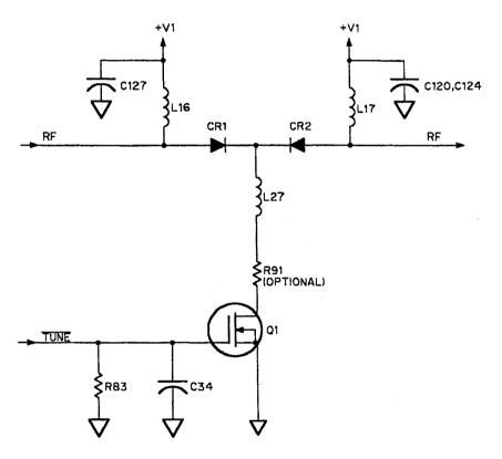
Figure 2-58. TUNE/NORM Switch, Simplified Diagram
