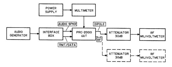
Figure 3-2. Test Set-up No. 2
