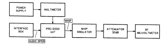
Figure 3-5. Test Set-up No. 5
