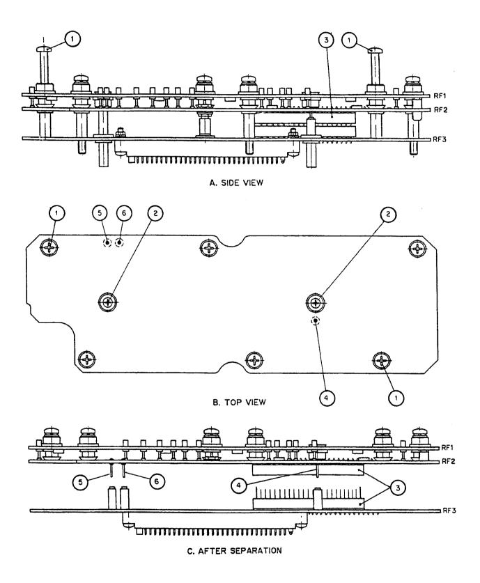
Figure 3-14. Modules RF1/RF2 and RF3 Assembly
