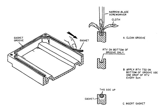
Figure 3-7. Gasket Installation
