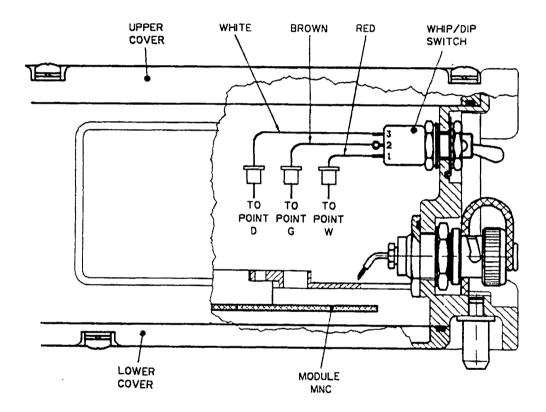
Figure 3-15. WHIP/DIP Switch and Wiring
