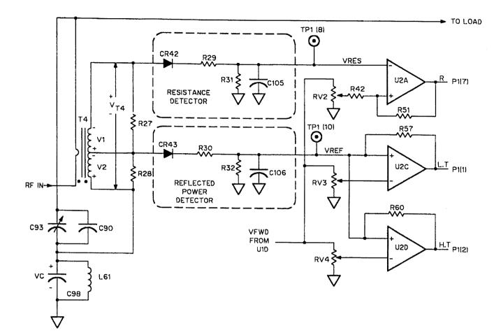
Figure 2-64. R and VSWR Sensors, Simplified Diagram
