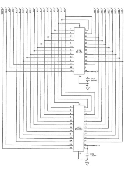
Figure 2-72B. Module MNC, Schematic Diagram (Sheet 2 of 2) 2-357/2-358
