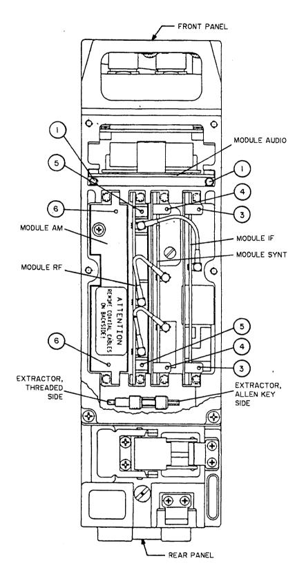
Figure 3-9.A. View on Modules Side (Sheet 1 of 2)
