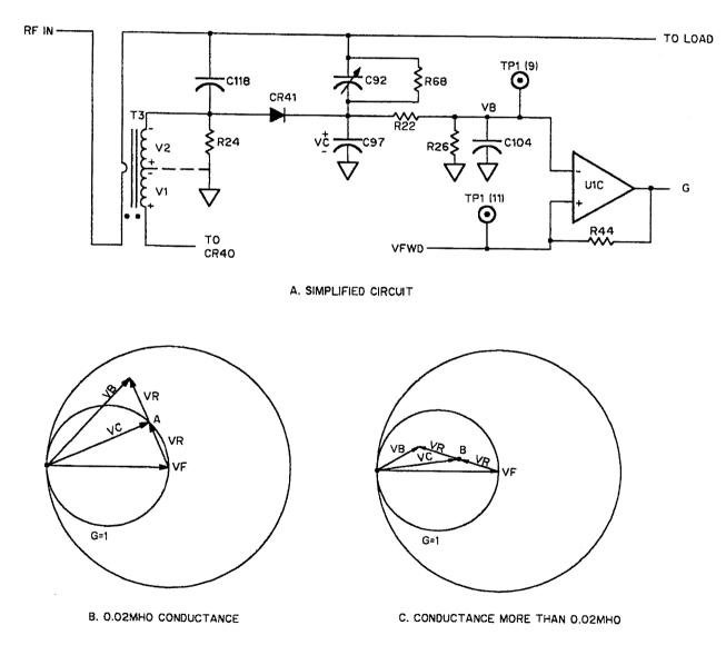
Figure 2-63. G Sensor Operation
