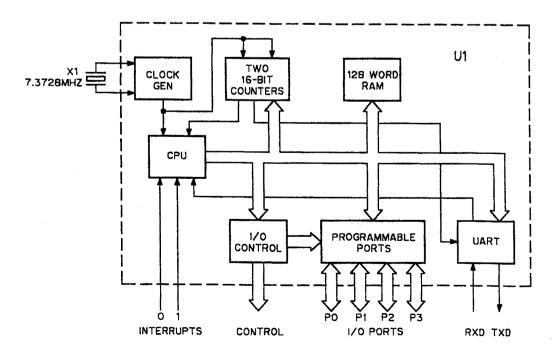
Figure 2-70. Module MNC, Microcontroller Block Diagram
