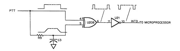
Figure 2-73. PTT Transition Detector Operation
