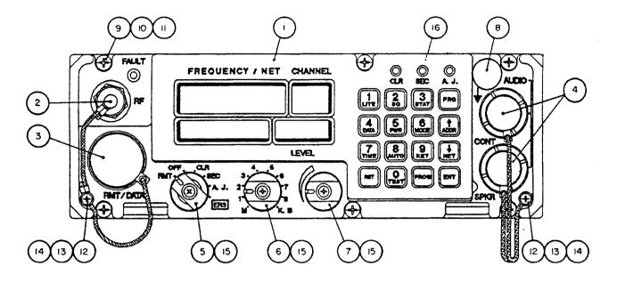
Figure 3-8. RT-2001, Front Panel Components
