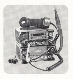
The ERC-310 Transceiver is a fully synthesized VHF-FM Manpack Radio that has been developed for cost-effective, reliable communications under combat conditions anywhere in
