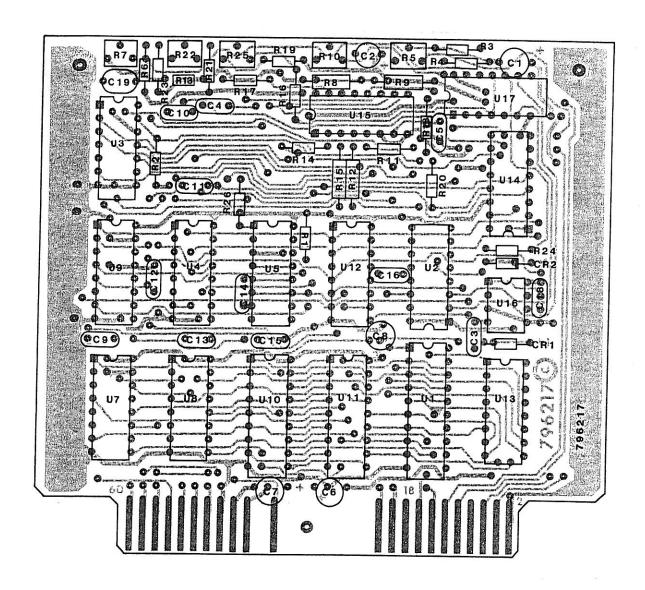
Figure C-1. Type 796217-1 Digital Refreshed Display (Option 2), Location of Components
