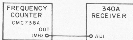
Figure 4-34. Test Setup, 1-MHz Oscillator Adjustment
